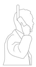
Stand outside with a clear view of the sky with the phone antenna pointing upwards. There must be a clear line of sight between the phone's antenna and the satellite.
