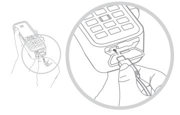
Connect the charger to a power source and the micro USB connector to the port at the base of the phone, under the USB/audio protective cover.
