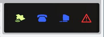
Iridium network. When the Iridium network is found and the ComCenter II successfully registers with it, the satellite icon will stop blinking and stay on solid, indicating the system is ready for use.
