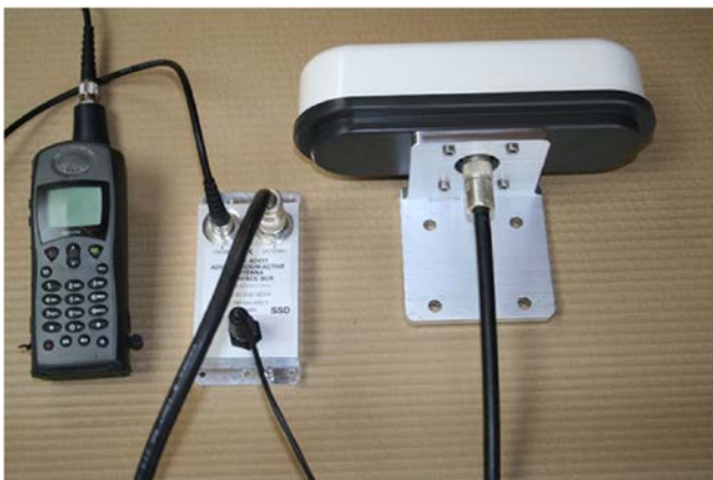
Figure 3. AD511-3 Power Break-In Box for use with +18 to +36 v DC supply.
