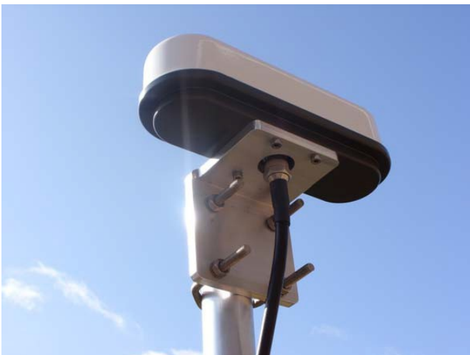
Figure 2. AD511-2 Active Iridium antenna with mounting bracket and coaxial down-lead
