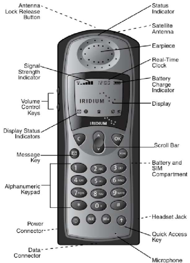
Note: Phone shown with antenna in stowed position.
