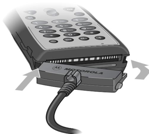
2. **Plug the travel charger** or auto accessory adapter into the appropriate power source. The phone beeps, flashes the
